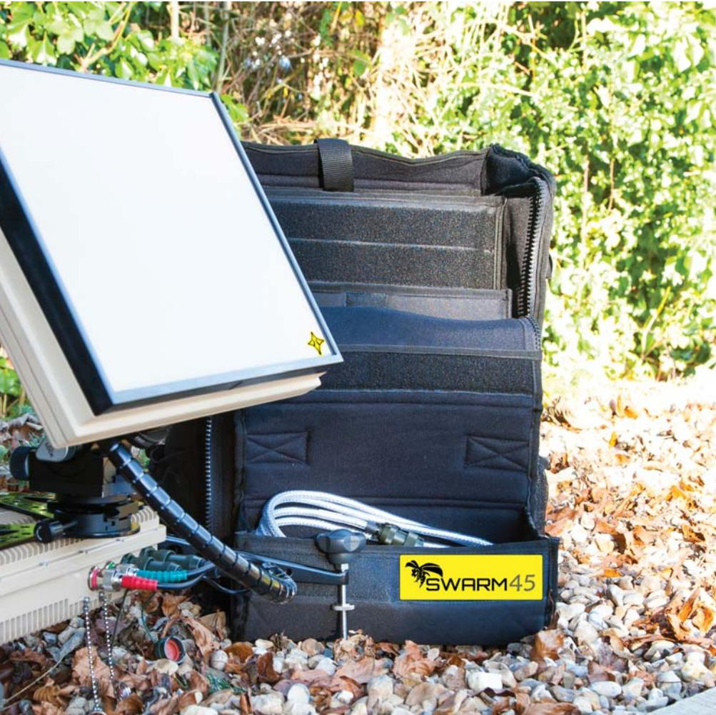
increased when using a flat panel antenna compared to a parabolic, as the signal passes through the antenna only once, reducing rain attenuation. Additionally, the flat panel design sheds water easily and avoids water pooling.”
